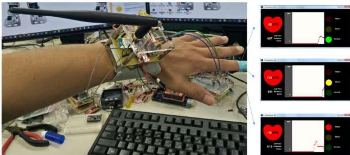
**Gambar 4.** Node Sensor Pulsa Berbasis LoRa 920MHz
