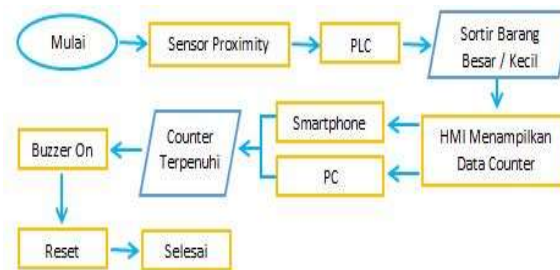
Figure 2. Flowchart of Operational Workflow and Real-Time Monitoring
