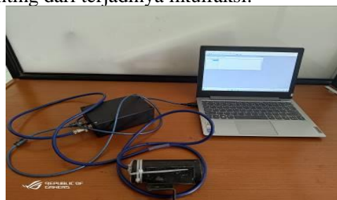
Gambar 3 Soil pore water pressure test equipment
